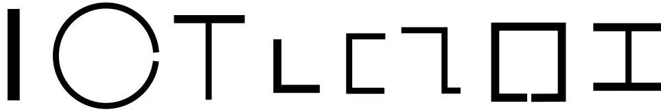
FIGURE 8.1. Open thin wall section examples.
